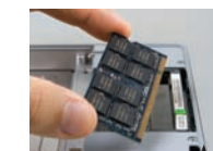
FIGURE 6-13 Result: RAM is a computer's equalizer and relatively inexpensive. On a laptop, you often gain access through a panel on the bottom. (Image: iStockphoto.com)
